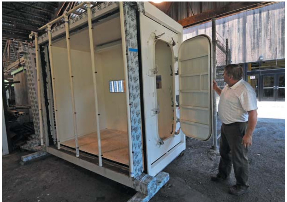
Glazier apprentices must test their skills in the "hurricane" booth. Simulated conditions with rain and wind up to 76 mph test a student's seal against the elements.
